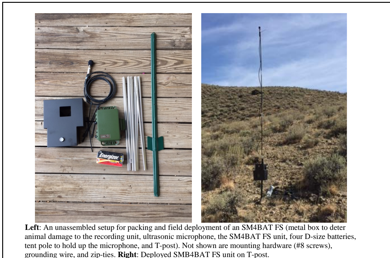
Figure 8. SM4BAT FS Acoustic Recorder Unit Set-up
